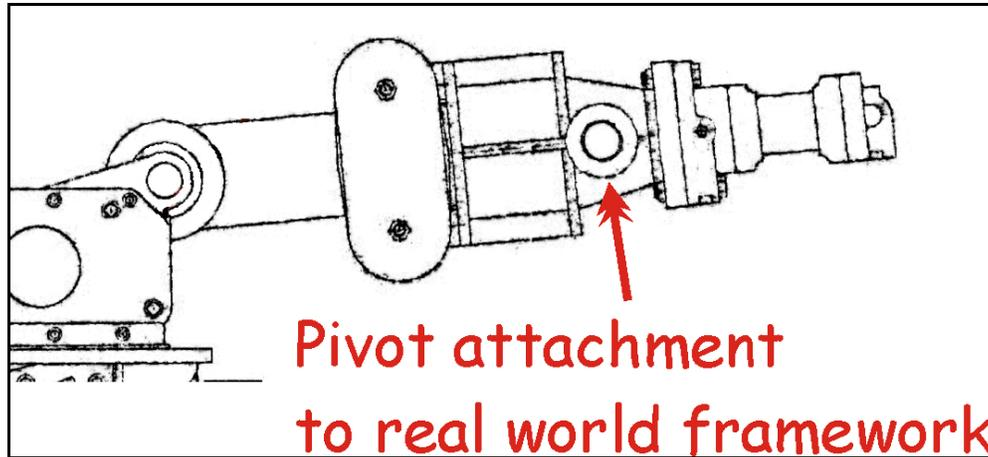
The picture above shows where the cradle attaches to the polar axle framework allowing for the adjustment of the cradle.
